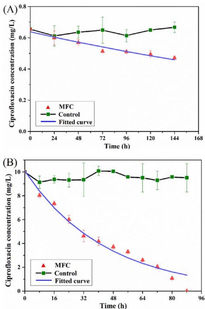
Fig. 1. Change in ciprofloxacin concentration during one cycle in the microbial fuel cells. (A) After operation for 1 month. (B) After operation for 1.5 years. The initial ciprofloxacin concentration was 10.0 mg/L. All the reactors were operated in batch mode. MFC indicates microbial fuel cell with electroactive biofilms. The control represents microbial fuel cell with abiotic electrodes.
