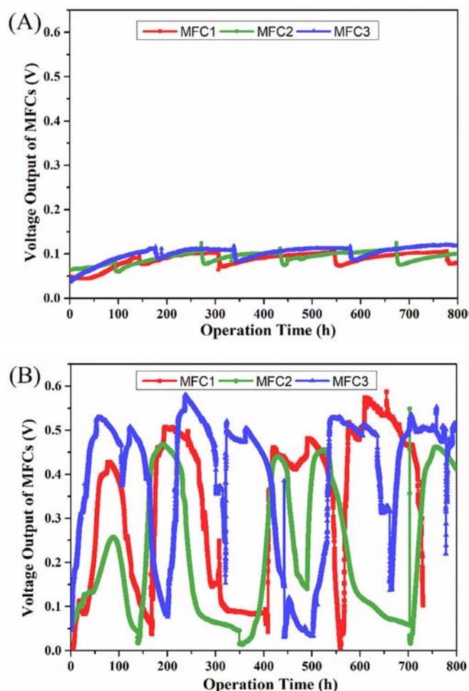
Fig. 2. Voltage output of microbial fuel cells (MFCs). (A) After operation for 1 month. (B) After operation for 1.5 years. MFC1, MFC2 and MFC3 are three biological replicates.
