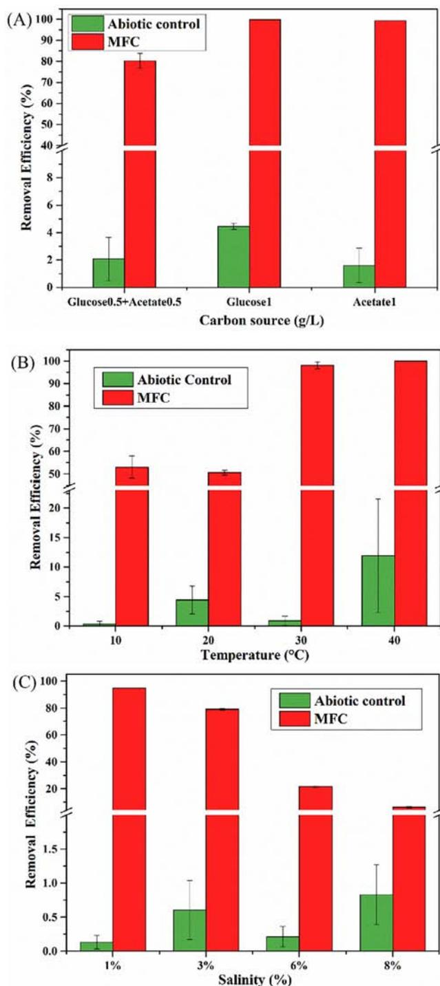
Fig. 4. Effects of environmental factors on ciprofloxacin removal. (A) Effects of carbon source on ciprofloxacin removal. Glucose 1 represents 1.0 g/L of glucose. The scale of break in the Y axis is from 10 to 40; (B) Effects of temperature on ciprofloxacin removal. The scale of break in the Y axis is from 23 to 45; (C) Effects of salinity on ciprofloxacin removal. The scale of break in the Y axis is from 2 to 4.
